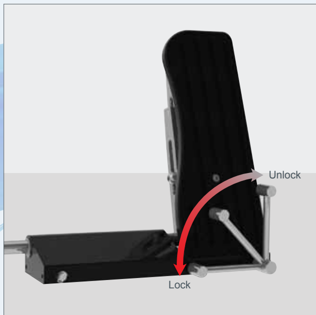
Quick release mechanism for easy removal of the LFA
