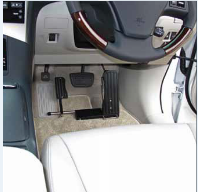
Left Foot Accelerator locked in position ready for operation.
